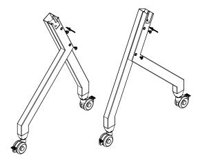
1. Secure forward and rear legs using (4) screw A and Allen Wrench A.
