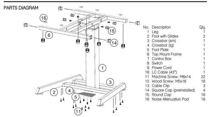
Lay out all components and hardware to ensure that you have all the components and hardware listed on the parts page.
